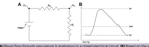
**Fig 4. (A)** Blood flow through vasculature is analogous to a closed electrical circuit. **(B)** Based on the same physics principles, BlueDop is able to measure the resistance and amplitude and calculate values like mean anklebrachial index (ABIm) through the validated pressure from flow algorithm.
